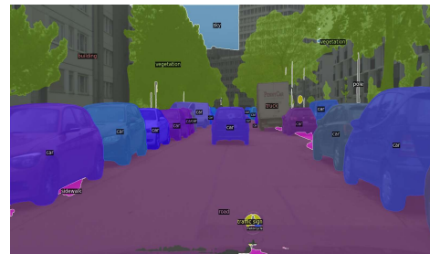
Fig 6. Inference using the pretrained Panoptic DeepLab model on Cityscapes dataset with inference time of 0.29 FPS
