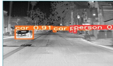
Fig 4. Inference using the pretrained YOLOv5 model on FLIR dataset with inference time of 50.07 FPS
