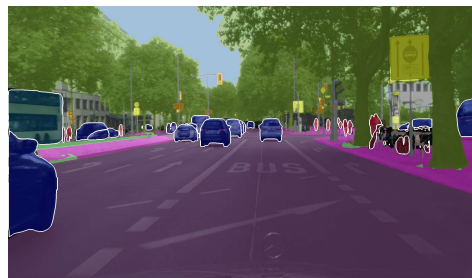
Fig 5. Inference using the pretrained EfficientPS model on Cityscapes dataset with inference time of 0.61 FPS
