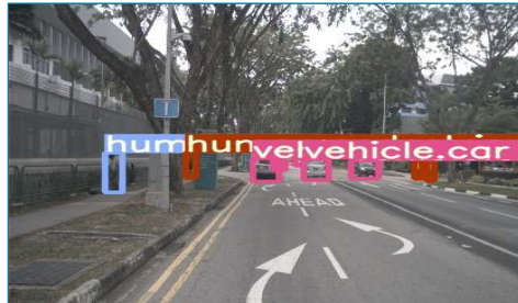
Fig 3. Inference using the pretrained YOLOv5 model on nulmages dataset with inference time of 54.55 FPS
